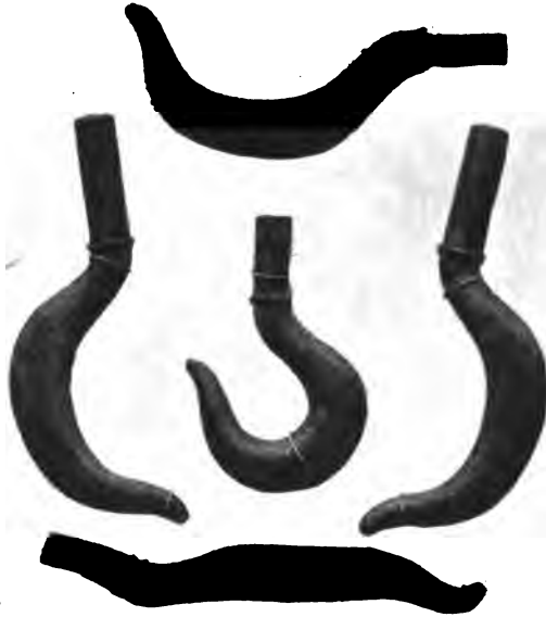
FIG. 377.—Crane Hooks and Results of Tests.
